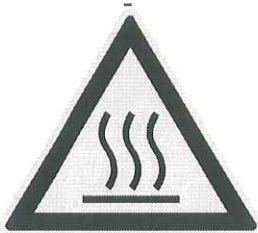
Warning about hot surface
