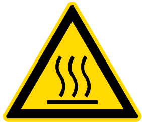
Warning about hot surface
