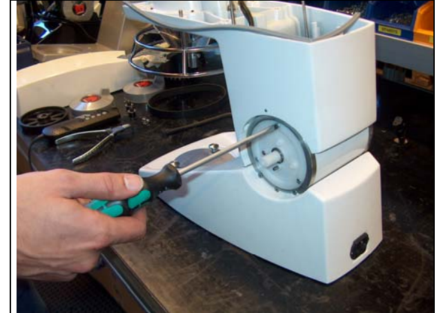
20. Loosen the three screws holding the tilt bearing.
