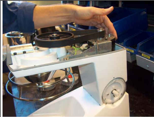
12. Push the motor forward in order to slacken the belt.
