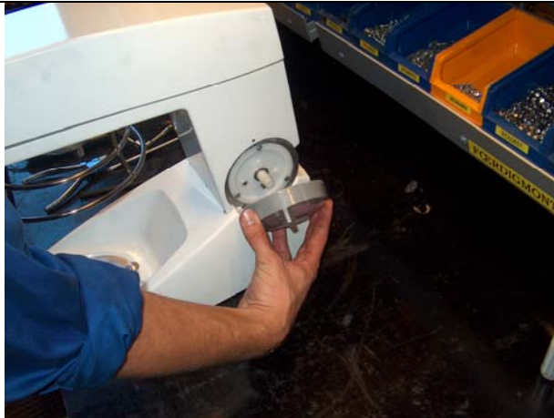
31. Close the mixer and reinsert the buttons carefully. See to it that they are correctly placed, not interchanging right and left.
