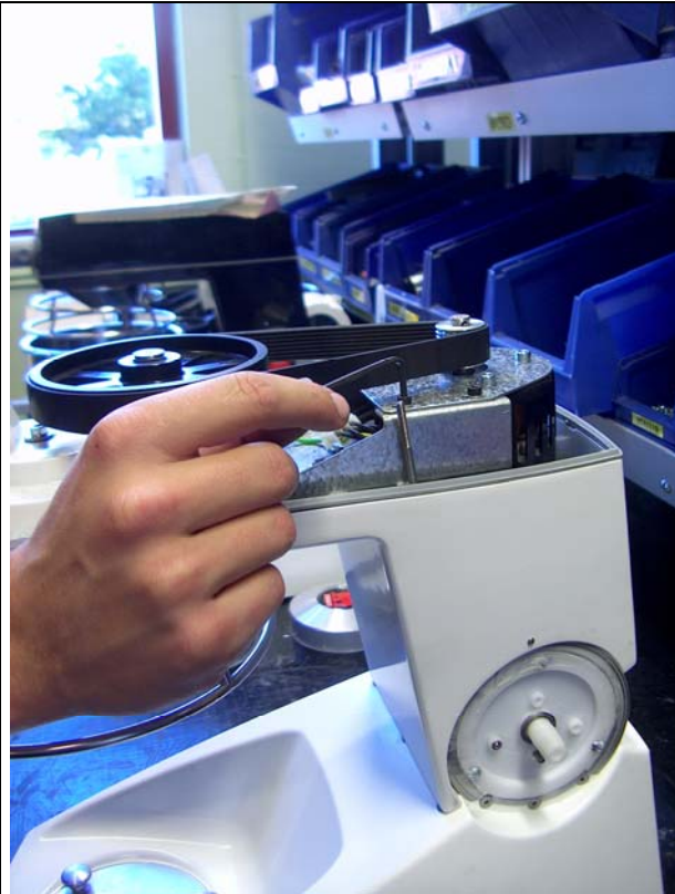
11. Loosen the 4 socket screws holding the motor.
