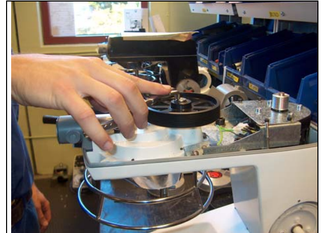
14. Remove the circlip holding the belt wheel.
