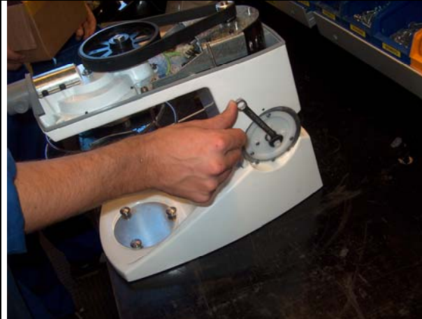
28. Use an 11 mm open-end spanner to open the mixer.
