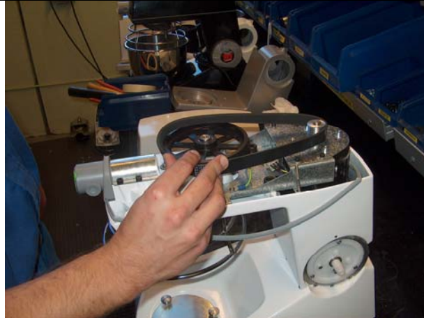
26. Mount belt wheel, circlip, and at last the belt.
