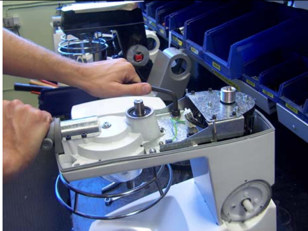
16. Loosen the two 10 mm socket screws.
