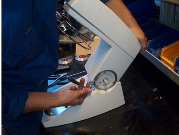
30. Tighten the hidden screws holding the lid.
