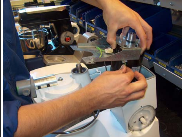
18. Lift the entire motor up with base. Gently pull the wire free.
