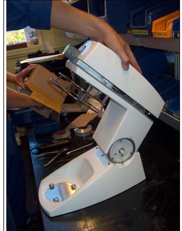
29. Reinsert the rubber gasket in the track and put the lid on the mixer. See to it that the gasket lies properly in both tracks. Also be aware of the gasket around the attachment drive.
