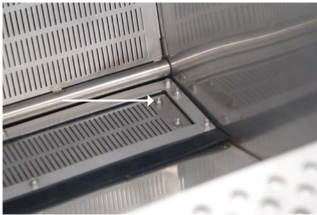
Nuts holding the damper.
