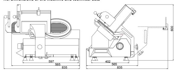
overall dimensions 728 x 565 x 600 mm counter space required 597 x 402 mm max. cutting size (blade 300 mm) app. 305 x 210 mm max. cutting size (blade 330 mm) app. 305 x 225 mm thickness of slices 0 - 25 mm (infinitely variable) Manufacturer: Hermann Scharfen GmbH & Co. Maschinenfabrik KG Ruhrstr. 76-76a, D - 58452 Witten, Tel. 02302/2827713/14
